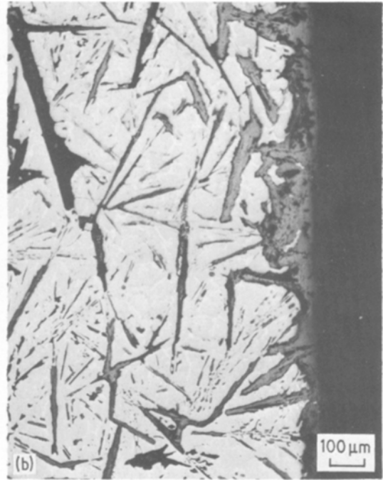
Figure 7 Optical micrograph of the carbide–oxide interface in a Ti–Cr–C composition containing 4.6 wt% retained chromium at several temperatures. Note the graphite “ghosts” next to the oxide film and the increasing pore size due to agglomeration with oxidation temperature.
